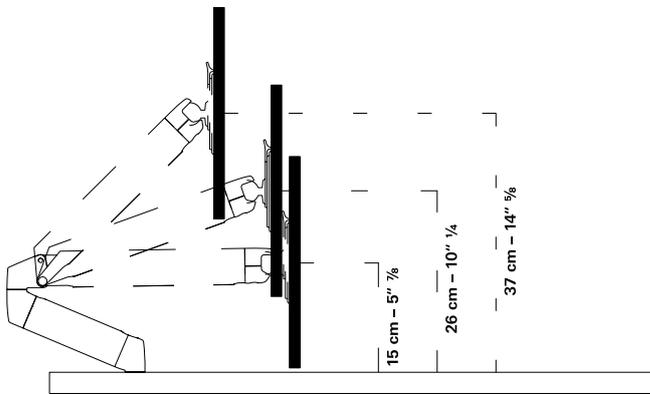
**HORIZONTAL EXTENSION OF THE DYNAMIC MONITOR ARM WITH SINGLE JOINT**
