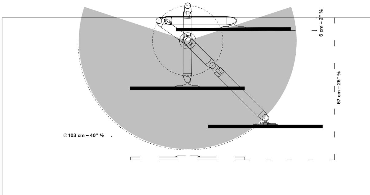
VERTICAL EXTENSION OF THE BASIC MONITOR ARM WITH SINGLE JOINT
