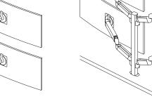
Vertical post (H46 cm) with two monitor arms and grommet connection to the table
