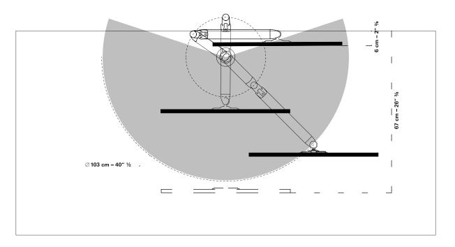
VERTICAL EXTENSION OF THE BASIC MONITOR ARM WITH SINGLE JOINT
