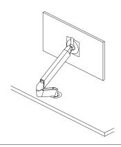
Basic monitor arm with double-joint and grommet connection to the table
