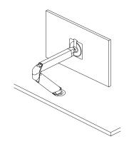
Dynamic monitor arm with double-joint and grommet connection to the table
